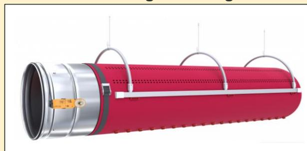
The FabricAir® VarioDuct™ features an internal membrane to separate the two airflows for heating and/or cooling purposes. This membrane is kept in place by the static pressure, thus does not flutter, providing the perfect airflow for each purpose; heating or cooling.
