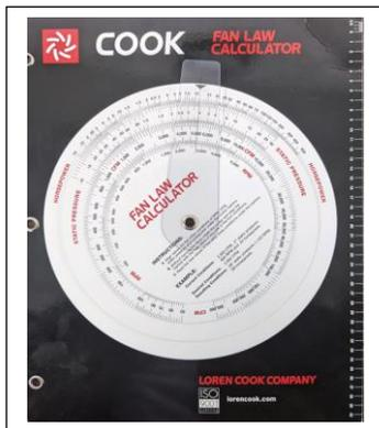
Looking at our example raising the CFM by 1,000 CFM would raise the static pressure to 4" and require a 15 HP motor operating at 2,700 RPM. But we still have a problem, the 15 HP motor will not fit. On the 110 MHA-HD. So, just to raise the CFM by 1,000 CFM will result in changing out the entire fan and increase in the motor HP dramatically.
